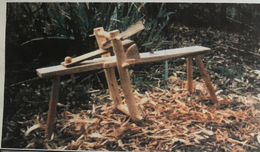
Shaving Horse - used in many crafts for shaving wood. A chair bodger will use one to prepare billets for turning on the pole-lathe.
